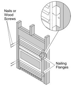
Figure 10 - Attaching Fireplace to Wall Studs
